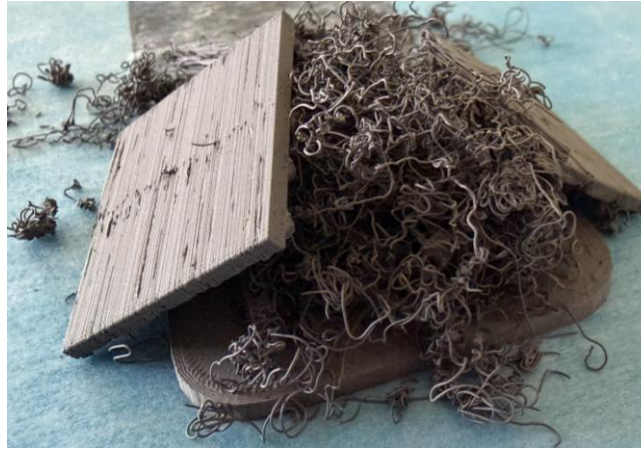
Figure 6.4 Defective lattice specimen illustrating the principal ADAM failure modes: partial blockage of the cellular volume by residual support material, localised strut collapse and fusion, and sagging of the upper sandwich plate
